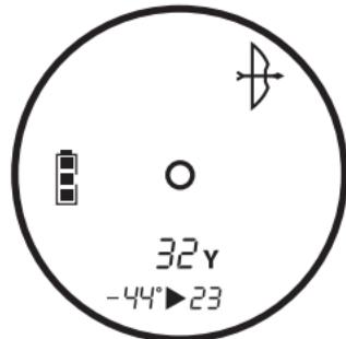
When line of sight distances from 7-199 yards are displayed, the Bow mode indicator will automatically be displayed along with angle and a compensated distance. If distances greater than 199 yards are displayed, the Bow mode Indicator will automatically turn off along with compensated distances.
